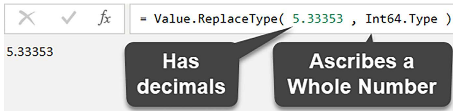
Figure 5.42: Incompatibility between the Type Claim and value
