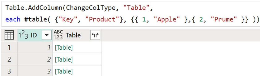
Figure 6.38: Creating a table value using the #table function
