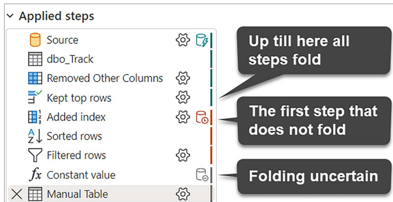
Figure 15.8: The query folding indicators signal the folding status of each applied step
