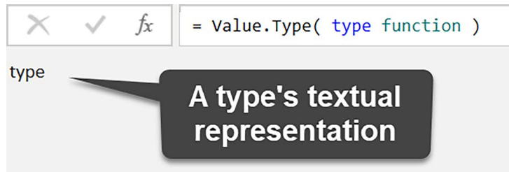
Figure 5.9: The Value.Type function returns the textual representation of a type
